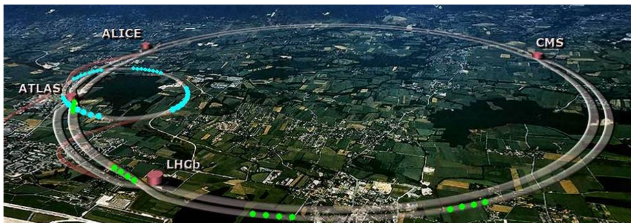
Figure 3.1: The Large Hadron Collider. The Super Proton Synchrotron accelerates the protons and feeds them to the LHC tunnel to collide at the interaction points of four experiments, ATLAS, CMS, LHCb and ALICE.
