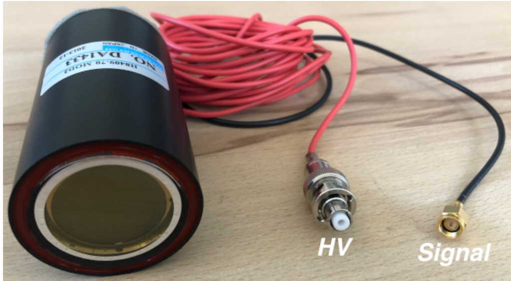
Figure 4.5: Photo of the Hamamatsu H8409-70 photomultiplier tube assembly with the display of the high voltage (HV) and signal cable.
