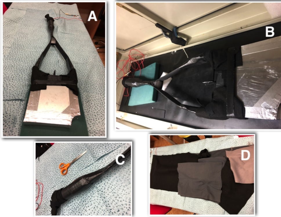
Figure 5.13: Pictures of the light-leak testing: display of the setup (A), module placed in a dark box (B), detail of the covered PMT (C), insulation against outer light (D).
