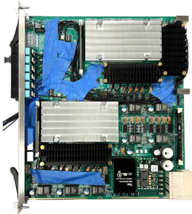
Figure 5.6: The GCMv3 prototype board with relevant components [33]. The blue tape secures cables close to the board to ensure proper insertion into the ATCA crate.
