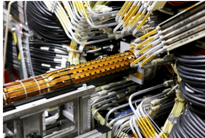
Figure 3.13: The insertion of the IBL sub-detector at the midpoint of its installation journey [25].
