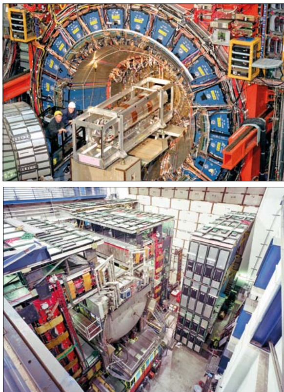
Fig. 1. CDF and DØ are complex, general-purpose detectors with over one-million detection channels. Four storeys high, they weigh in excess of 5000 tonnes. (Image credit: Fermilab.)
