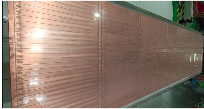
Figure 4.1: One strip layer, for a Long-shaped RPC, horizontal strips (bending plane).
