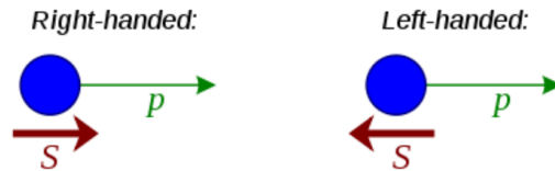
Figure 1.5. Example of right-handed and left-handed helicity [23].
