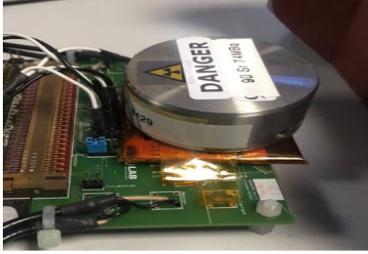
(a) The setup for ^{90}\text{Sr} source
