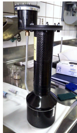
Figure 1: L_6D_6 detector filled with C_6D_6 liquid scintillator.
