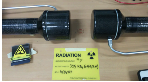
Figure 4: Experimental set-up: the two detectors are facing the radioactive source. I collected data for two detectors at the same time.
