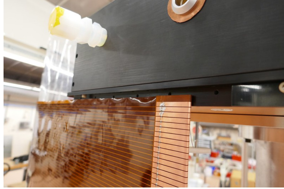
Figure 3.13: Image of FTPC2 field cage and resistors and gas connections during assembly.
