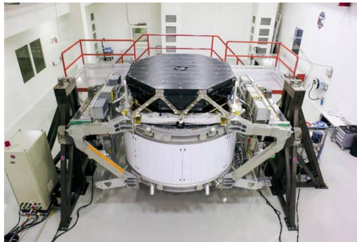
Figure 6.1: AMS-02 at CERN in December 2007. The entire detector is read out by a flexible network of independently operating slave computers and one out of four main DAQ computers of AMS-02 as the master.
