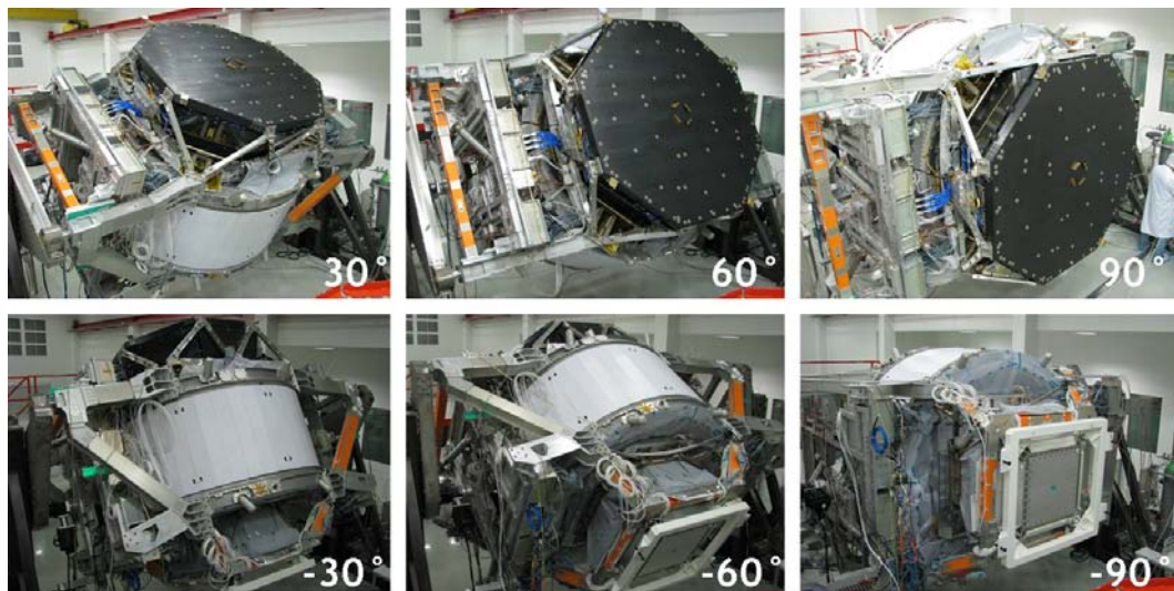
Figure 7.26: AMS-02 rotation test at the end of the pre-integration phase. The main aspect was the test of the mechanical stability mainly of the tracker. The position of the ladders was monitored throughout the test by the tracker alignment system (TAS).
