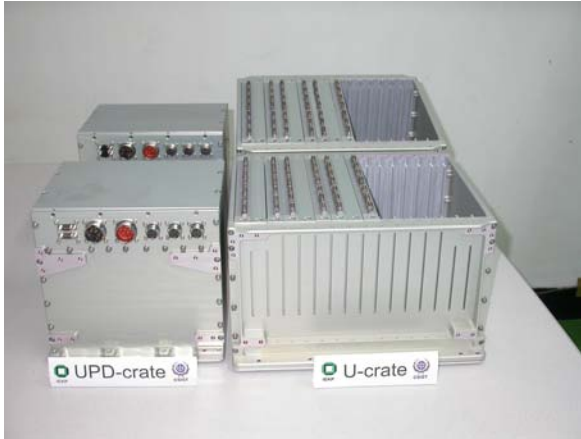
Figure 5.10: U-crates during the assembly. The crates are partially equipped with electronics boards, which are slid into the corresponding slots into VME connectors on the backplane. Before the backplane has been mounted to the backside of the crate's aluminum walls.
