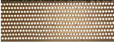
Figure 3.15: ECAL fibers embedded in 640 kg of lead arranged in 18 layers.
