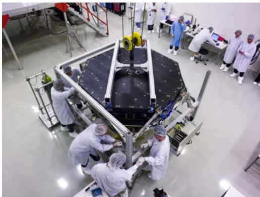
Figure 7.23: Lifting operation of the TRD during the pre-integration phase.
