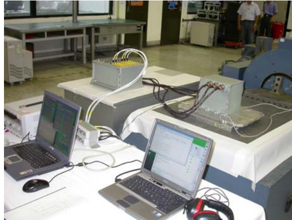
Figure 5.17: FM ESS vibration table test setup. The UPD box is mounted on the shaker table to be vibrated in horizontal Y-direction. It is powered and connected to the U-Crate throughout the test. The test software verifies a failure free operation before, during and after the test.
