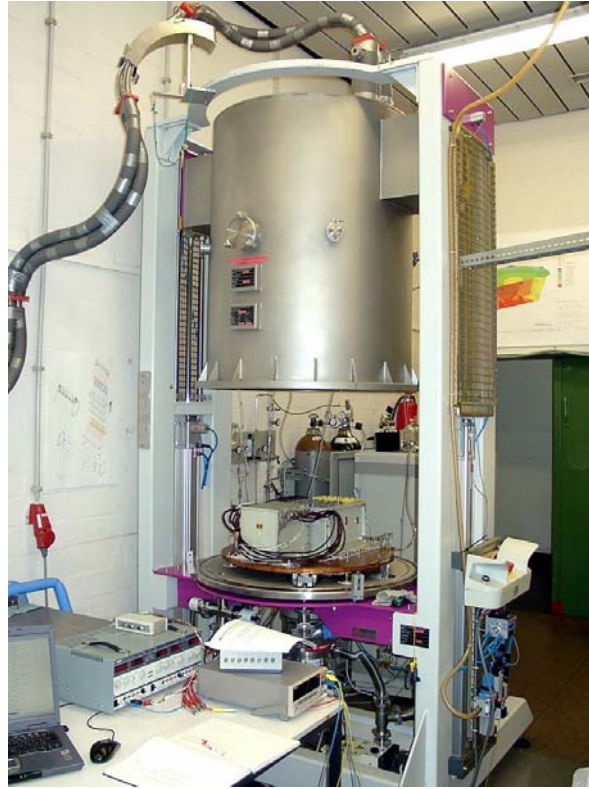
Figure 5.18: Thermal vacuum chamber at RWTH Aachen. The chamber is able to accommodate one U-Crate and one UPD box. Three UFS boxes are mounted in front of the U-Crate not yet done in the picture.
