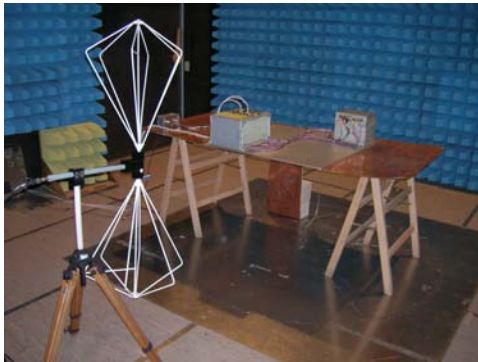
Figure 4.32: Emitted electromagnetic radiation test. The antenna records the emitted radiation during the operation of the U-Crate.
