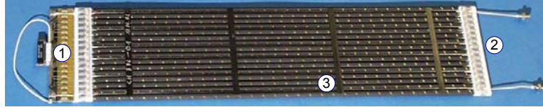
Figure 3.20: A TRD straw tube module. The 16 tubes are connected to the \text{Xe}/\text{CO}_2 gas circuit by a manifold (2). On the opposite side the tube end board (1) is attached, which connects the high voltage and decouples the signal by 16 capacitors from each straw tube. Additional carbon fiber stiffeners (3) are glued between the tubes.
