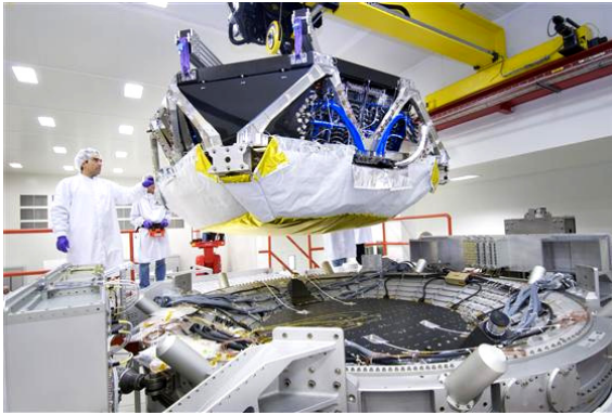
Figure 5.24: Lifting of the TRD to be mounted on top of AMS-02.
