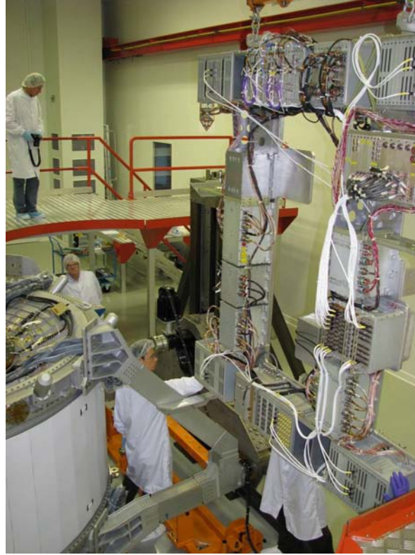
Figure 3.35: Picture of the partially equipped RAM radiator during the pre-integration phase in 2007.
