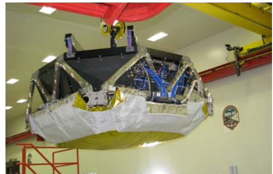
Figure 3.22: The assembled TRD lifted by a crane. The carbon fiber structure is stabilized by the M-structure machined from solid Aluminum.
