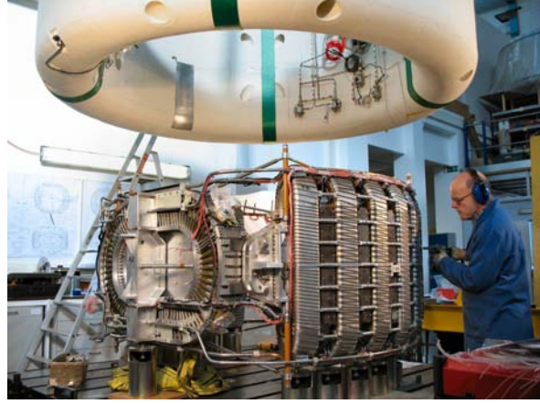
Figure 3.8: The coils of the superconducting magnet and the Helium tank. Both will be embedded in the AMS-02 vacuum case.
