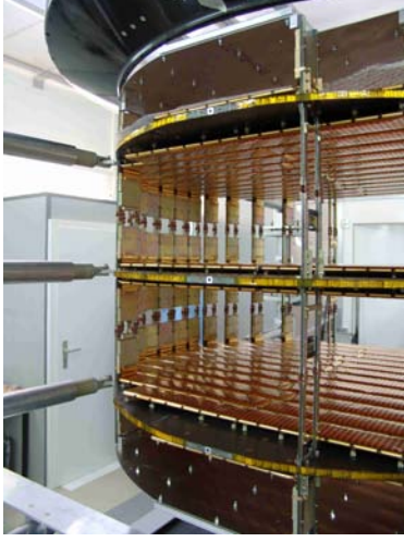
Figure 3.4: The six layers of the AMS-02 tracker mounted in its transport frame. The top and bottom layer are mounted separately on the top and bottom cover of the tracker.
