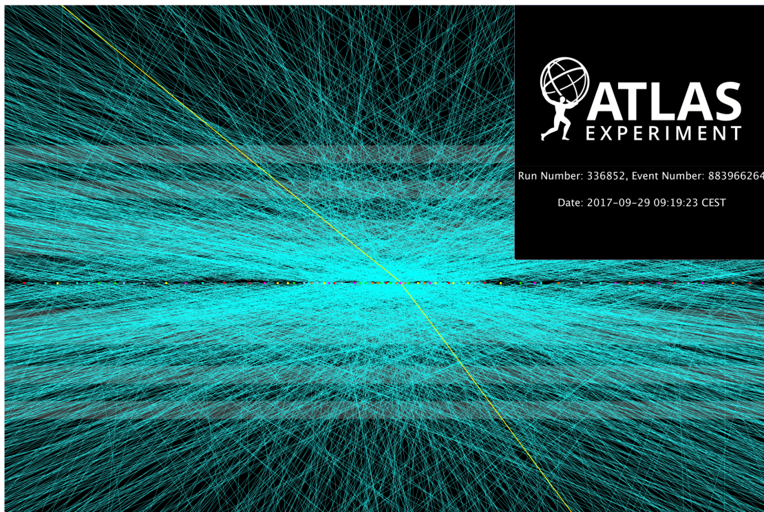
Figure 3.1: A display of Z \rightarrow \mu\mu candidate event from pp collisions recorded by ATLAS with LHC stable beams at a collision energy of 13 TeV. The Z boson candidate is reconstructed in a beam crossing with a pile-up of \mu = 65 . Tracks with p_T < 100 MeV are shown, with the two muon tracks highlighted in yellow. The large number of pile-up create a more challenging environment for reconstructing the hard scatter vertex. ATLAS Experiment ©2020 CERN.
