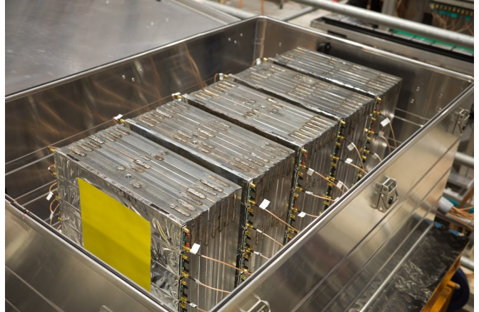
Figure 7.35: ECAL (left) and HCAL (right) prototype built and operated in TB4. The beam comes from the right.
