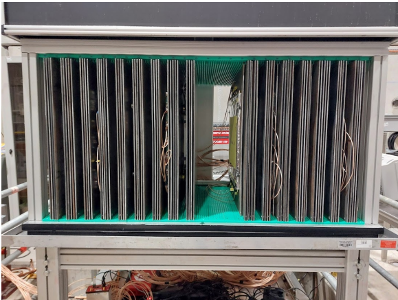
Figure 7.35: ECAL (left) and HCAL (right) prototype built and operated in TB4. The beam comes from the right.
