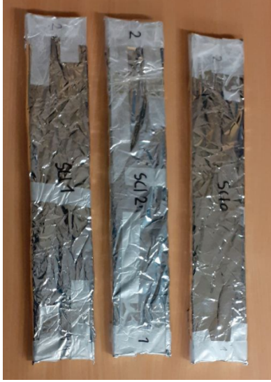
(a) Picture of the three scintillator bars used for the measurement in crumpled foil.
