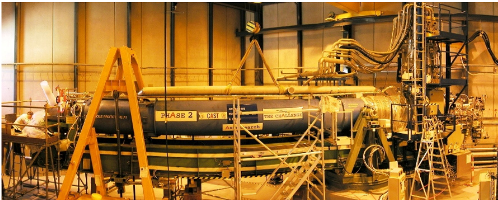
Figure 2.14: A picture taken during the installation of the expansion volume on top of the CAST magnet.
