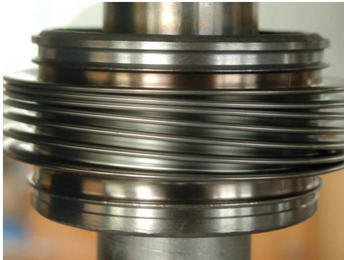
Figure 7.4: In plane squirm of nested bellows
