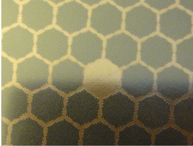
Figura 3.13: Cross-section of multifilamentary NbTi/Cu composite wire
