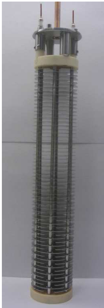
Figure 2.5: BLM ionization chamber introduced for the LHC. Metallic enclosure removed.
