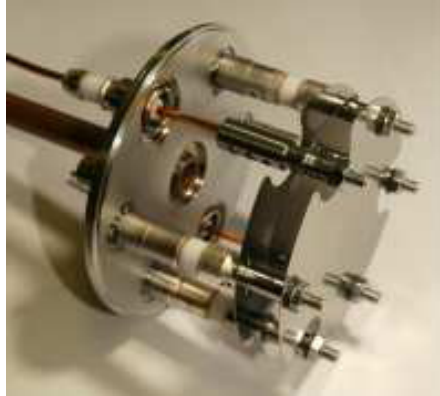
Figure 2.7: Secondary emission monitor. Metallic enclosure removed.
