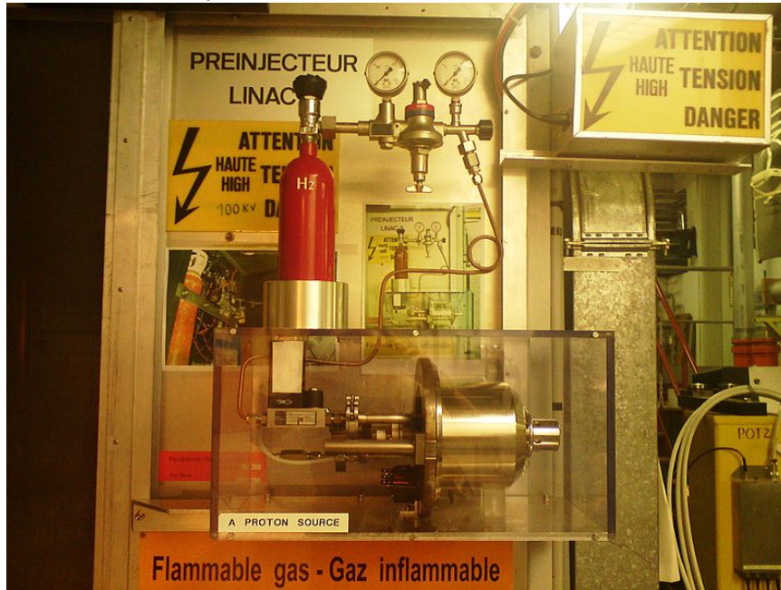
Figure 2.2: The red bottle contains hydrogen gas that is used to supply protons to the Linac 2, and ultimately, the LHC.
