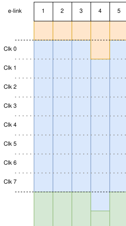
Figure 4.5: Diagram showing a single e-link, with index 4, which is late sending data to the lpGBT. Each colour corresponds to different data packet.
