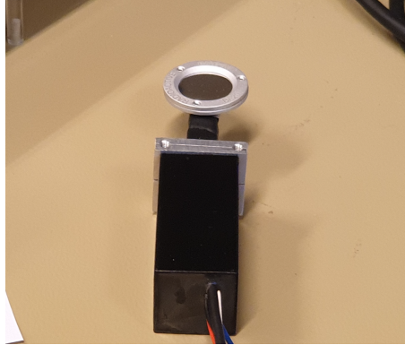
Figure 5.11: Photograph of ^{207}\text{Bi} source used for tests, placed above a scintillator and PhotoMultiplier Tube (PMT).
