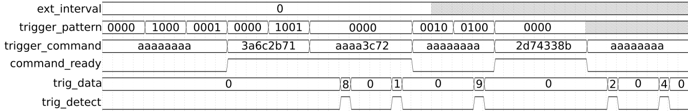
Figure 5: Simplified waveform diagram of the process of generating trigger patterns
