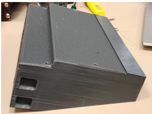
Figure 2.1.6: Side view of 3D printed version of Green Box.
