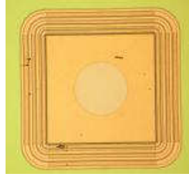
Fig.3.17 Picture of a diode with total area of 6 \times 6 \text{ mm}^2 and 4 contactable GR's structure (LAL design)
