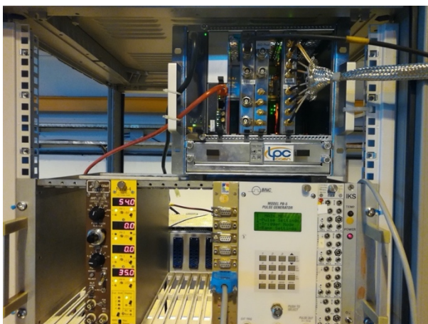
Figure 56. FASTER Acquisition system and high voltage power supply used in the ^{32}\text{Ar} campaign.
