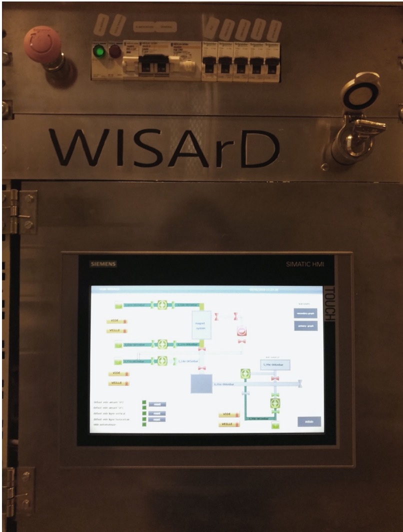
Figure 52. WISArD SIMATIC touch panel control. In the touch screen, the layout use to visualize the vacuum system through the beamline. Security measures are also shown in the picture.
