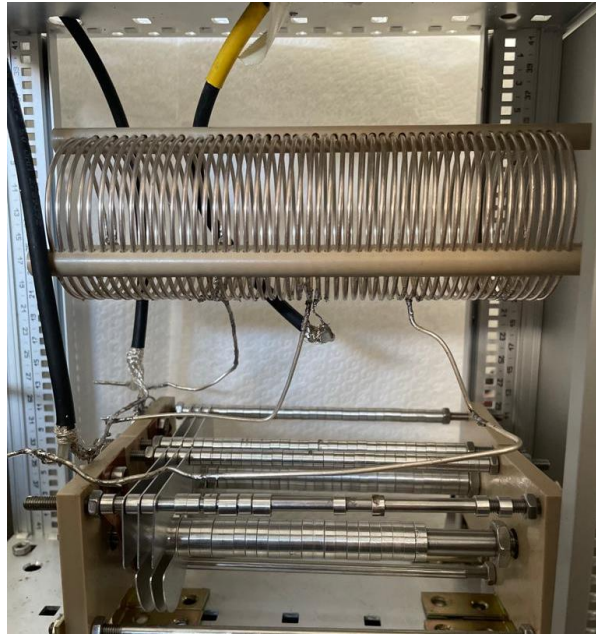
Figure (10): mockup design designed to test different resonance frequencies.
