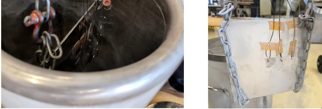
Figure 10. Absorber suspended from chain during the cold down (left) and the warming up (right)
