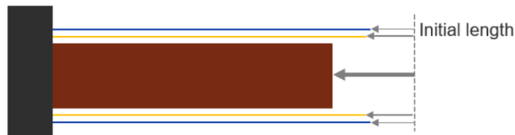
Figure 3. Free contraction of the absorber layers
