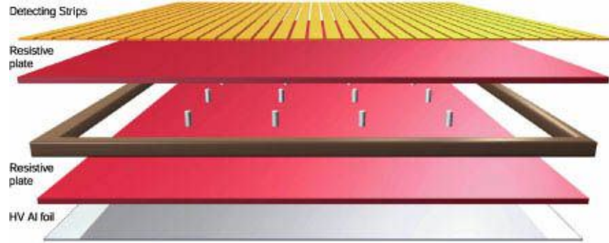
FIGURE 4.3: Resistive plate chamber (RPC) [26].
