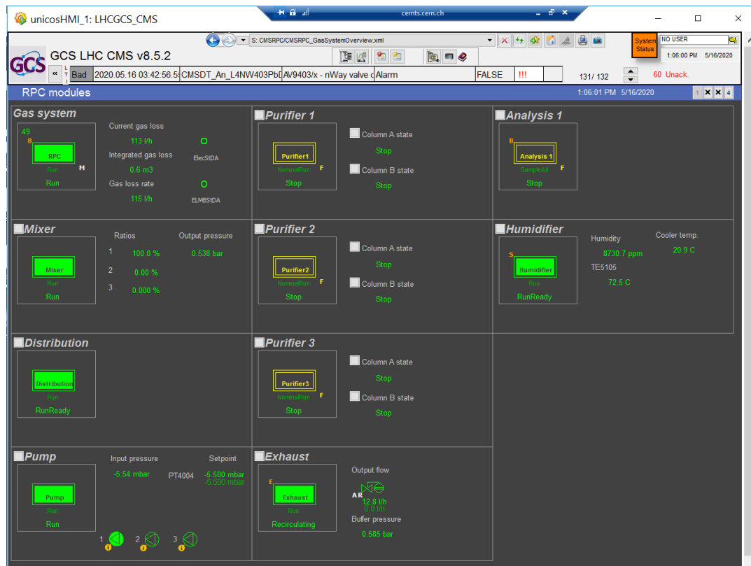
FIGURE 2.3: Example of WinCC-OA interface for the control and monitoring of a gas system
