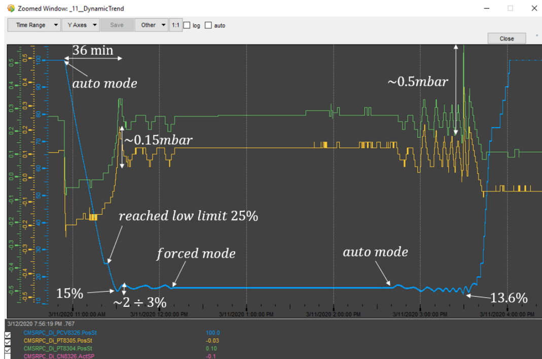
FIGURE 4.50: ASCO DN20 valve in auto mode (1)
