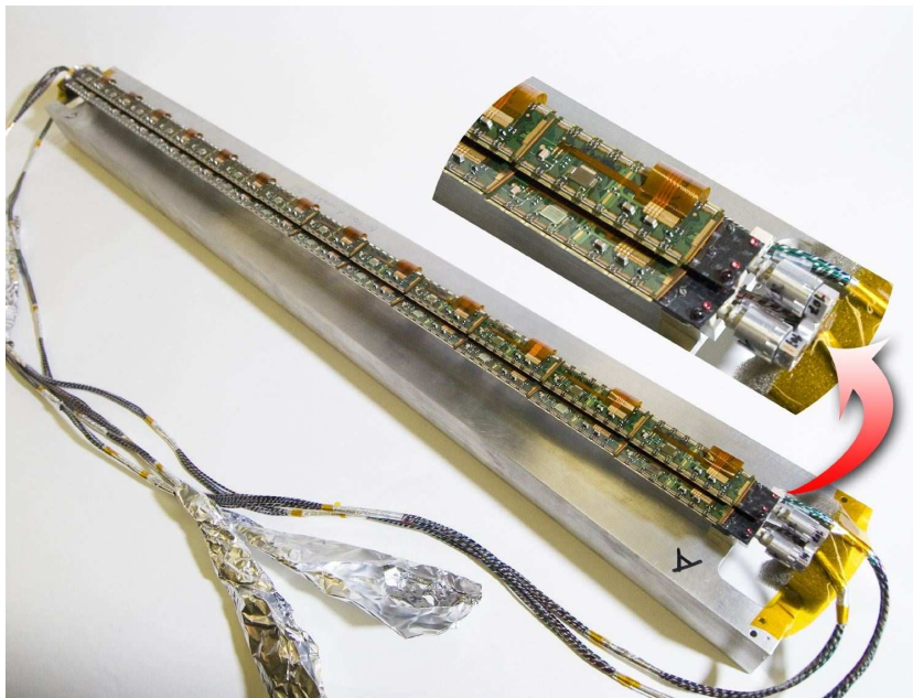
Figure 3.6: Detail of a bi-stave loaded with pixel modules.
