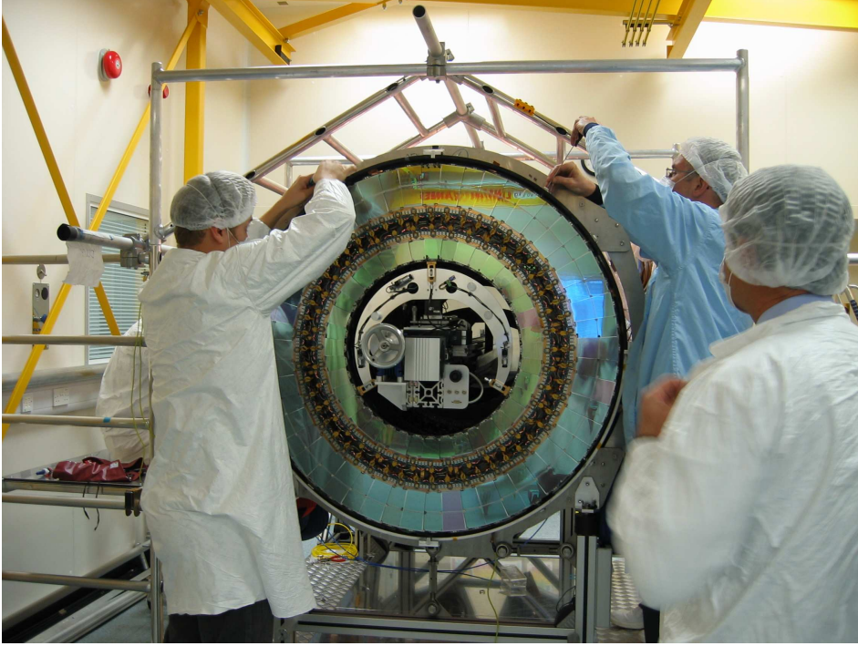
Figure 3.23: Photograph during the assembly of one SCT End-Cap (Liverpool, UK).
