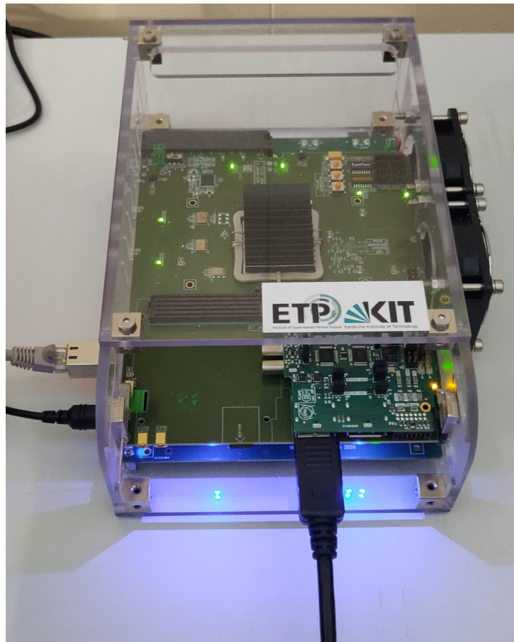
Figure 3.10: The FC7 board operated on the nano-crate. An custom FMC card allows the electrical communication with the ROC through a Display-Port cable.
