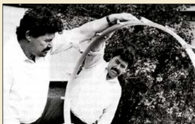
An inflatable mirror made from an aluminised mylar membrane 25\ \mu\text{m} thick, which has been developed at the CERN West Workshop. By varying the pressure applied to the membrane the mirror takes up varying quasi-spherical forms. The focal length can thus be varied for use in a Cherenkov counter.
