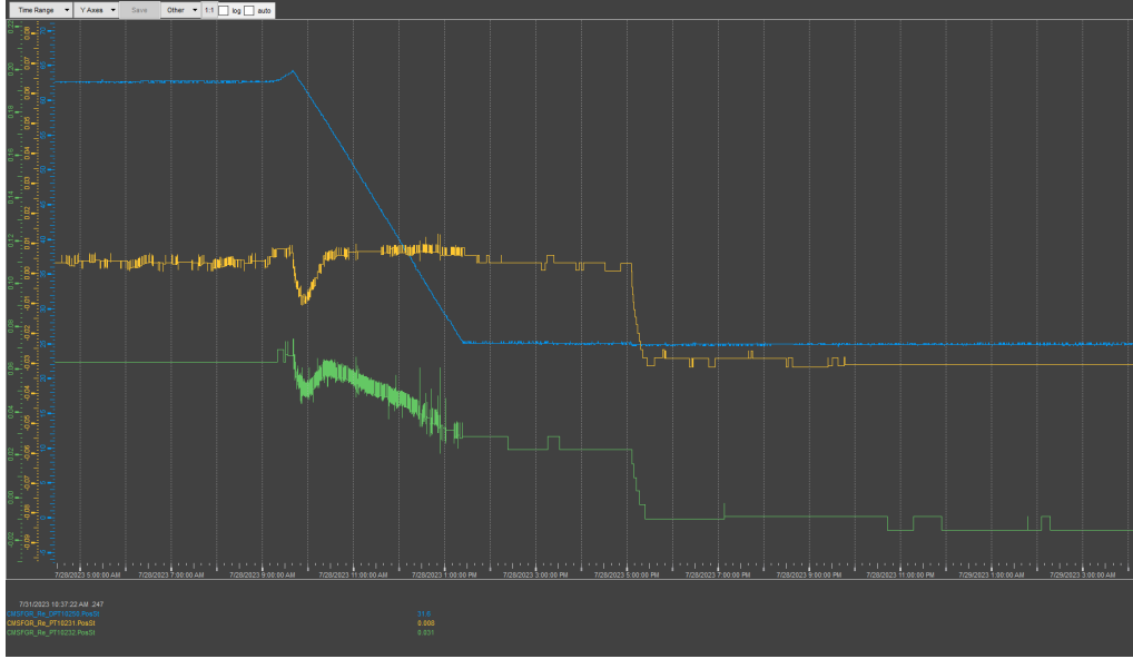
Figure 76: Column 1 pressure trends during the emptying phase. During the emptying phase, the liquid level (blue) starts decreasing, the yellow ( P_{top} ) and green ( P_{bot} ) curves have a minimum due to the perturbation for the compressor activation. After a transient phase, P_{top} reaches the Zimmerli setpoint and P_{bot} decreases with a similar trend of the DPT (blue).
