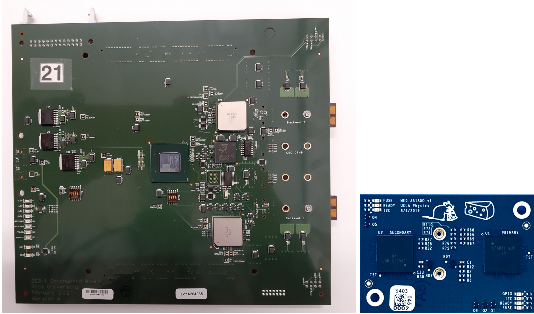
Figure 3.8: Pictures of the GE2/1 (left) and ME0 (right) OptoHybrids.
