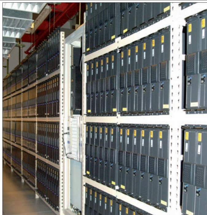
The Pion cluster at Fermilab consists of 520 Intel Pentium PCs.
