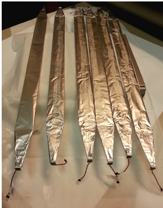
Figure 3.9: Scintillation detectors, ready to be built into the experiment. The assembly in figure 3.8 has been expanded by the SiPM boards depicted in figure 3.7 (b) and an aluminium wrapping.
