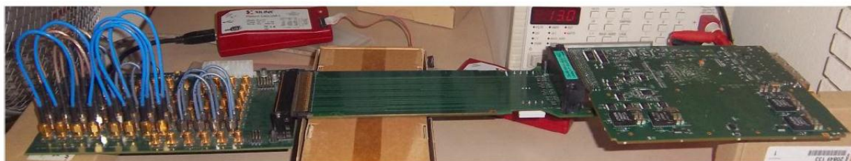
Figure 2-10: AMC high speed serial connectivity test setup 2.
