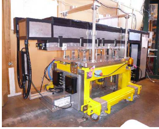
Figure 2.2: Photo of one set of ZDC calorimeters on the movable platform on the surface.
