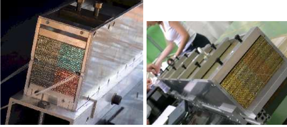
Figure 2.3: Front face of neutron (left) and proton (right) calorimeters.
