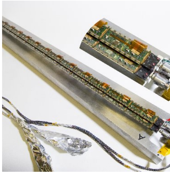
FIGURE 2.9: half-shell structure of the ATLAS pixel detector.
