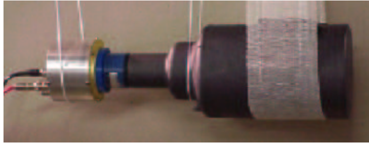
Figure 3.4: Neutron sensitivity optimized C_6D_6 detector.
