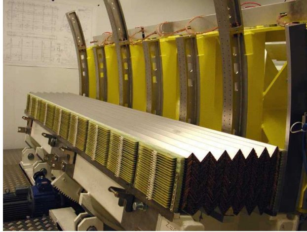
Figure 4.4: Photograph of a partially stacked barrel electromagnetic LAr module, where the accordion geometry is visible [57].
