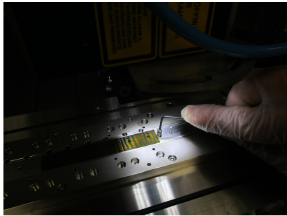
(e) Removing the support pins
