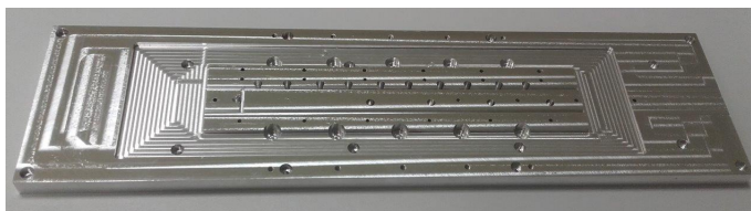
Figure 3.1: Mechanical Structure which holds the FPC
