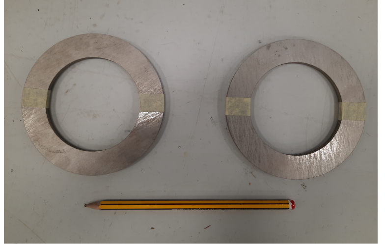
Figure 4.4: Left: Split-coil permeameter. Right: Toroidal ARMCO® Pure Iron Grade 4 material specimens.
