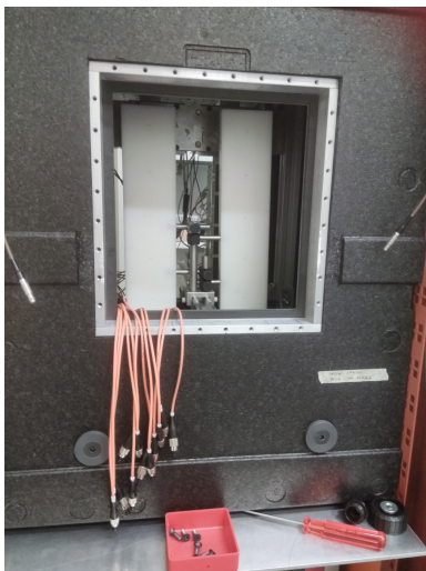
Figure 9: The back side of the SIN measurement setup. The orange cables are plugged into the Teflon boards to provide uniform illumination from the laser onto the MaPMTs, which are mounted directly behind them.
