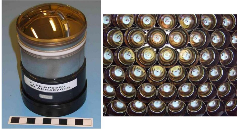
Figure 4.5: Left: single HPD, the ruler is 10 cm long. Right: Panel of HPDs inside RICH.
