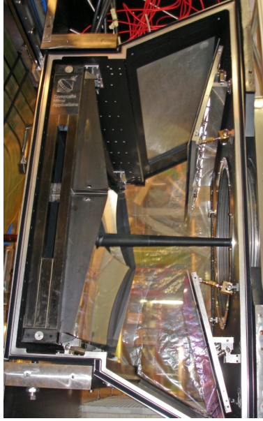
Figure 4.3: Picture of the RICH1 gas enclosure containing the flat and spherical mirrors (the interaction point is on the right). Also the beam-pipe crossing the detector is visible.
