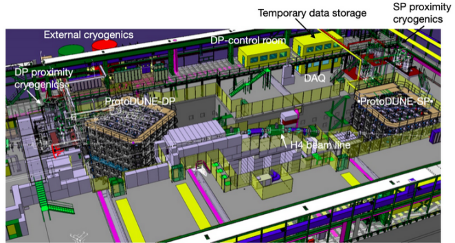
Figure 1: Layout of the EHN1 experimental area. The Dual Phase cryostat is on the left, and the Single Phase cryostat is on the right. Image source:[1]
