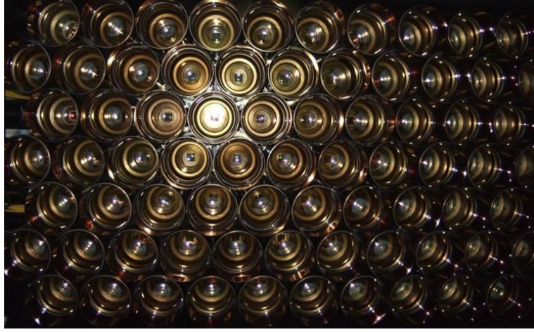
Figure 3.5: Photograph of the array of RICH 1 HPDs.
