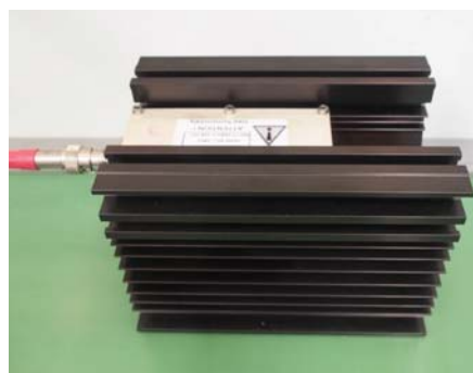
Figure 5.4. Diconex 18\ \text{kV} , 50\ \Omega , 160\ \text{W} terminating load.
