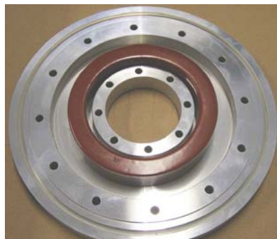
Figure 5.2. An aluminium bottom flange of the prototype adder with a Vacuumschmelze W567 magnetic core.
