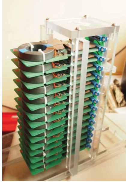
Figure 2.13. Photo of a series switch stack comprising 15 FETs [57].
