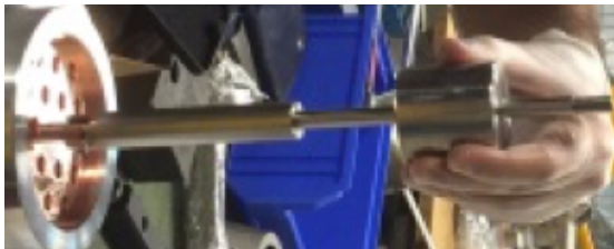
Fig. 6.4 Slide-hammer used to push and pull the tuning studs. The weight is thrown to either end of the shaft to deform the cavity wall [134].
