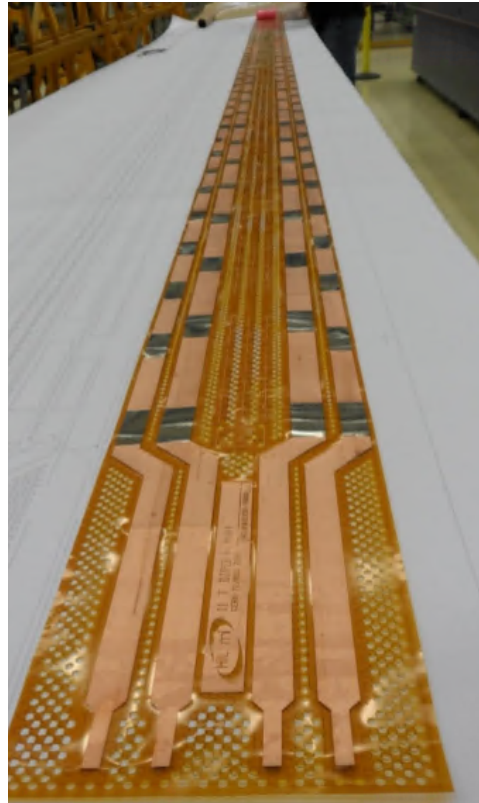
FIGURE 1.11: Quench Heaters strips of the 11T dipole [23].
