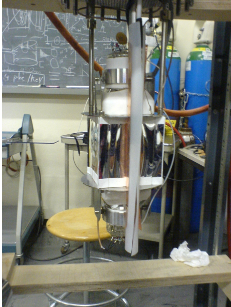
Figure 6: Open setup with mounted reflectors (shiny and reflecting surface with white borders)
