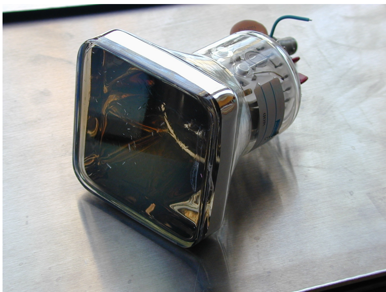
Figure 9: Technical Data of the Hamamatsu R6237-01mod photomultiplier
