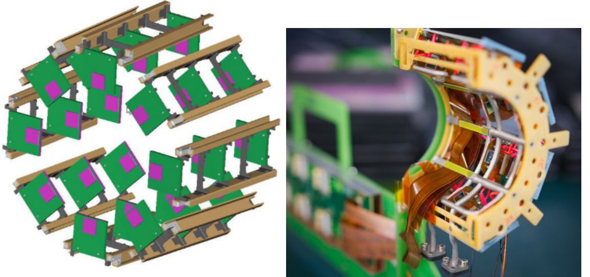
Figure 1.7. Left: Schematic image of the Pixel Luminosity Telescope (PLT) showing eight sets of three pixel detectors forming eight telescopes. Figure from Ref. [15]. Right: Photo of four PLT telescopes ordered to a quadrant with mounting support and connections to the readout electronic visible. Figure from Ref. [17].
